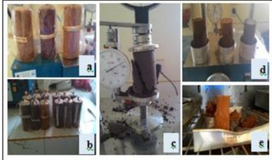
Figure 2: The stage of testing: a) the manufacture of the test object, b) curing process, c) testing of compressive strength (UCS test), d) weighing the specimen after testing, e) drying in an oven
